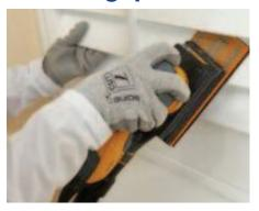
Mirka now has an extension pad to enhance the versatility of the Mirka® DEOS 353 CV 81x 133. The pad's overhang will enable users to sand further into corners and hard to reach areas.
